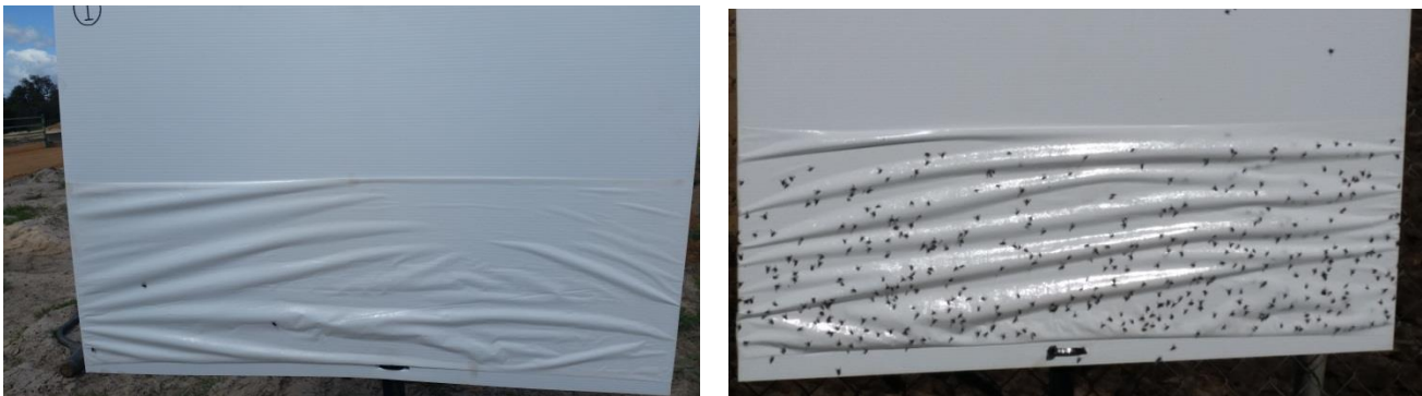
Fig. 3. Sticky film monitoring board with white sticky film before (L) and 30mins after exposure (R) where captured stable flies can be seen on the sticky film
